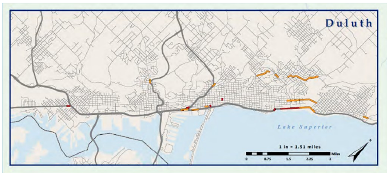
Forecast congestion for 2040: orange represents LOS E and red represents LOS F. Source: Connections 2040 by Duluth-Superior Metropolitan Interstate Council.
